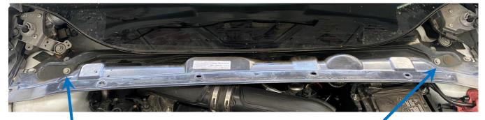
5. Remove 2 bolts holding the metal cover support & remove piece from engine bay.
